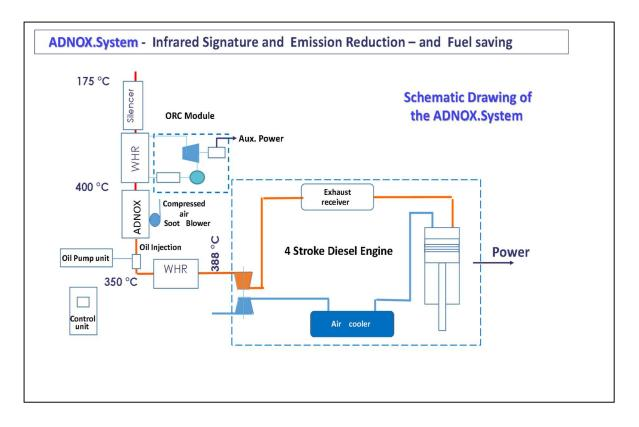
The heat recovered is used in an ORC plant for production of Power – hereby saving fuel and reducing the CO<sub>2</sub> emission.
